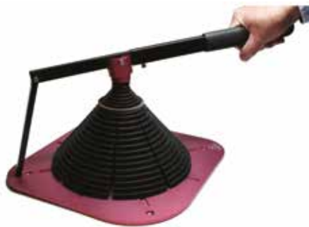
3. Extend the PTFE ring using 19SEAL STRETCHER . (diameters from 40 up to 250 mm).
