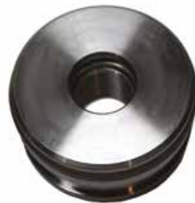
6. The PTFE seal is now assembled.
