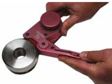
5. Calibrate the seal using the tool 19SEAL CLASPER . (diameters from 50 up to 360 mm).
