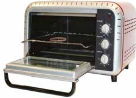
2. Heat the PTFE ring to a temperature of 120°C.
